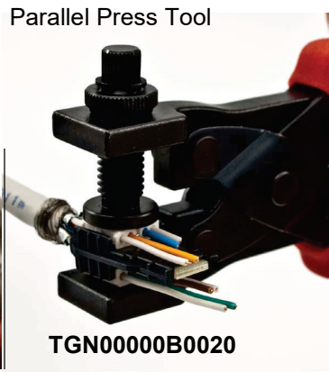
Cut all 8 wires using cutting pliers, wires protruding max. 0,5 mm
